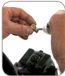
Add sealant and screw reducer into lubrication point
