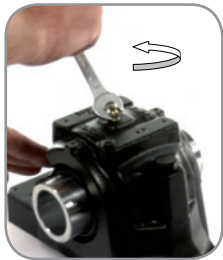
Clean lube-point and remove grease fitting
