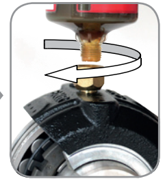
Screw lubrication system into lube-point
