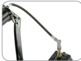
Prefill lube-point and any grease lines / connections (use the same grease that is contained in the lubrication system)
