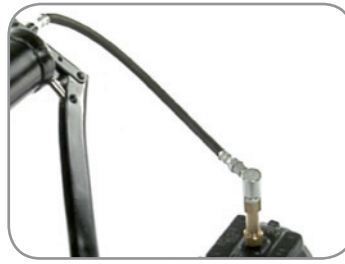
Prefill lube-point and any grease lines / connections (use the same grease that is contained in the lubrication system)
