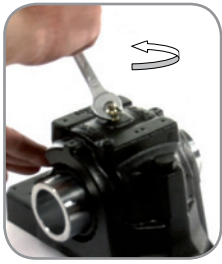
Clean lube-point and remove grease fitting
